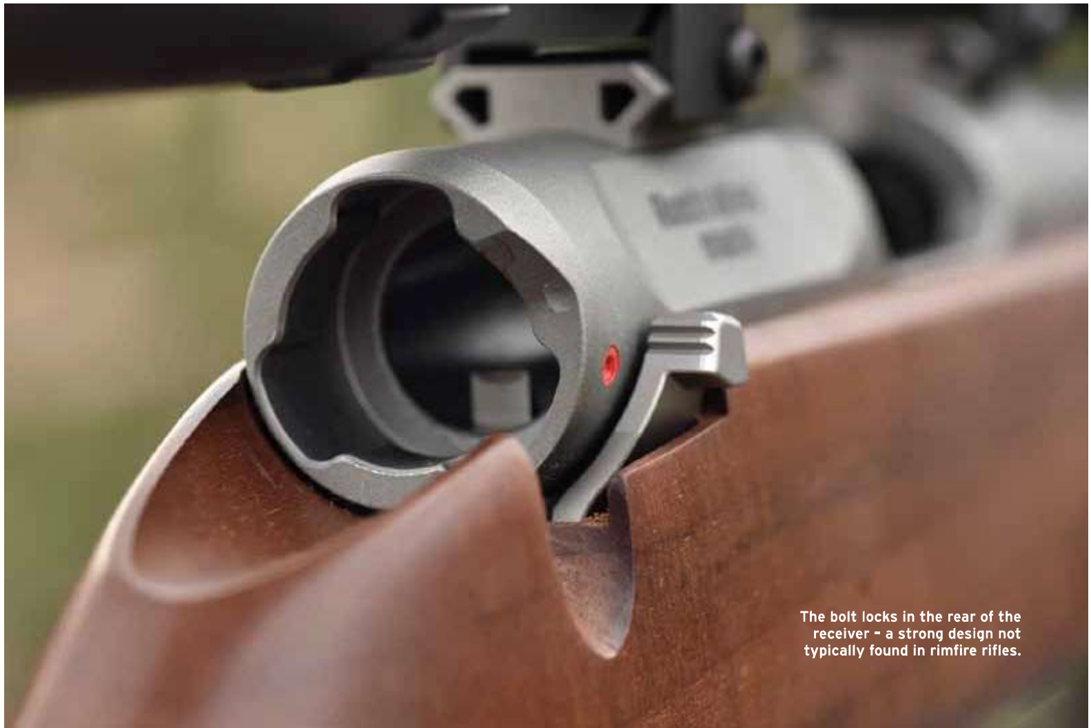
The LA 101 Crossover has a two-position safety, which allows the bolt to be opened with the safety engaged.
