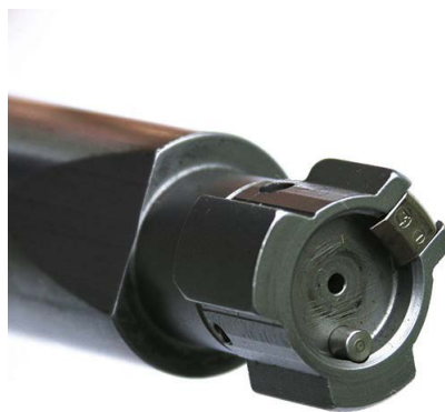
The bolt face showing the recessed face, the plunger ejector and the claw extractor set up in the locking lug.
