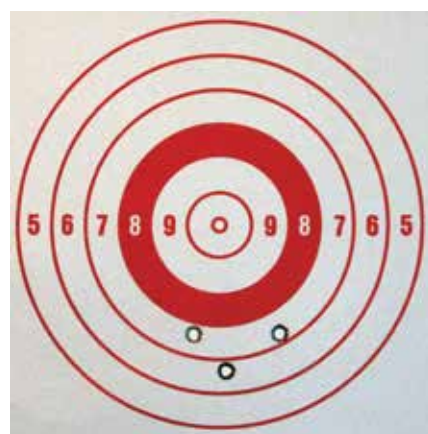
A 25mm group shot using the Winchester Super X load, a 40gn FMJ projectile at 1910fps.
