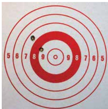
The best 100m group with the WMR LA101 measured 17mm. It was shot using the Winchester Supreme 30gn JHP load at 2250fps.
