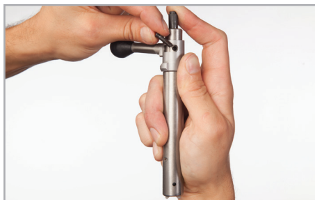
Figure 29: Bolt Handle Alignment
