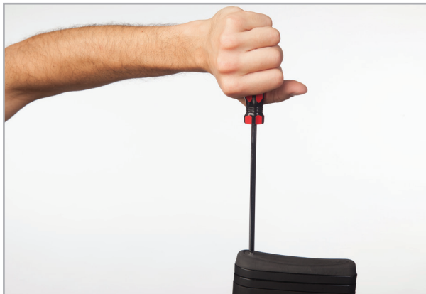
Figure 22: Length of Pull Adjustment
