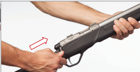
Figure 11: Closing the Action
