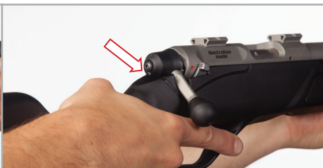
Figure 13: Rifle Uncocked or Fired
