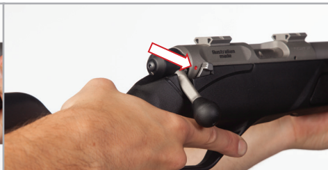
Figure 16: Safety Catch set to Fire
