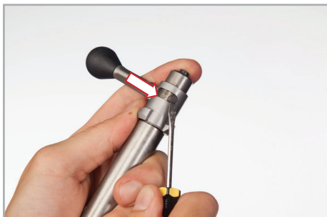
Figure 25: Bolt handle Retaining Pin
