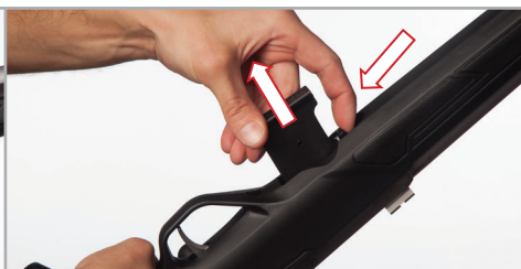
Figure 20: Removing a Magazine
