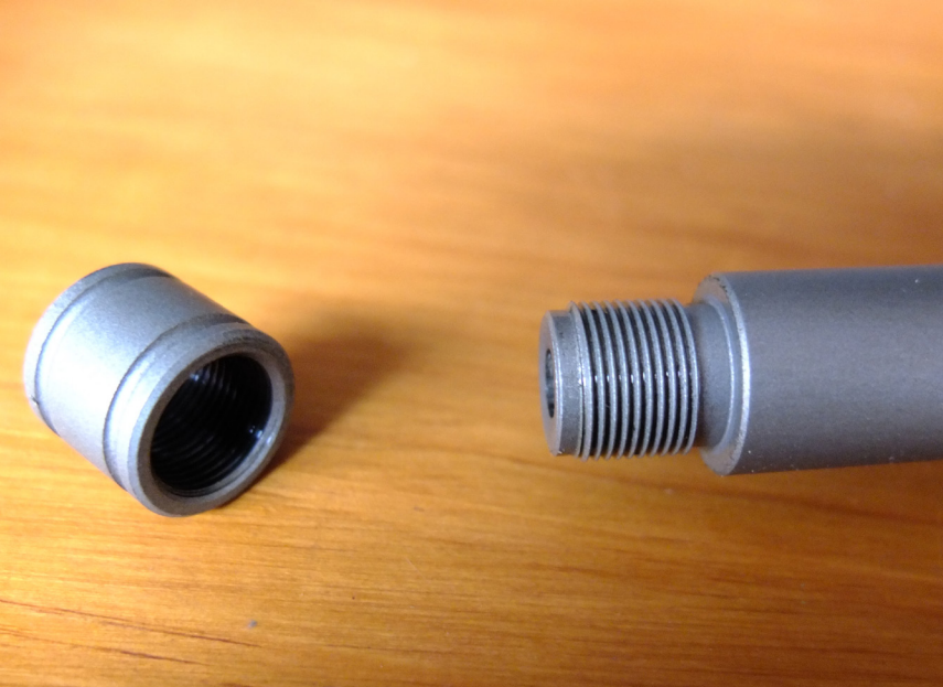
A false tip can be unscrewed from the end of the barrel to expose thread to fit a muzzle brake, or sound moderator.
