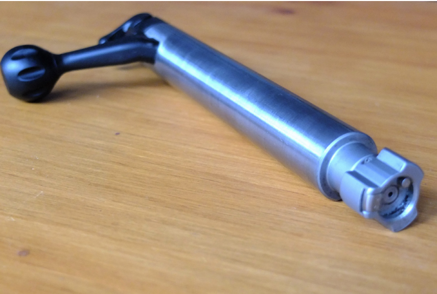
Precision finished full diameter bolt with knurled handle and three locking lugs.
