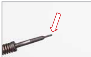
Figure 25: Firing Pin Nose
