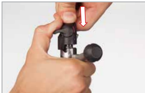
Figure 28: Bolt Shroud Insertion
