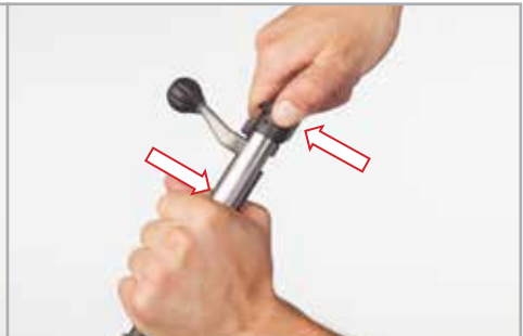
Figure 24: Bolt Shroud Removal
