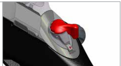
Figure 15: Safety Catch set to Safe (Bolt Locked)
