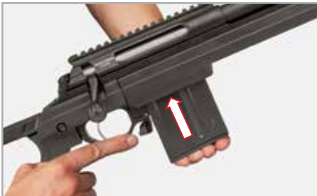
Figure 19.2: Fitting a Magazine (LA105 Woomera with XRAY Chassis Shown)
