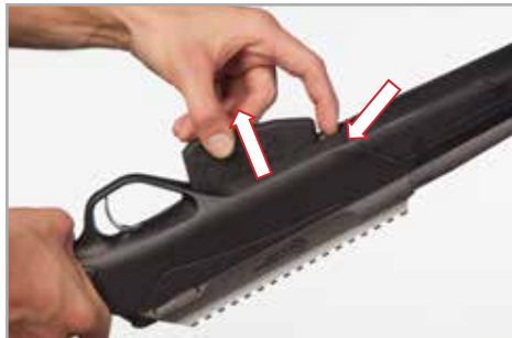
Figure 4.1: Magazine Removal (LA102 CrossOver with Polymer Stock Shown )
