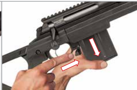
Figure 4.2: Magazine Removal (LA105 Woomera with XRAY Chassis Shown)
